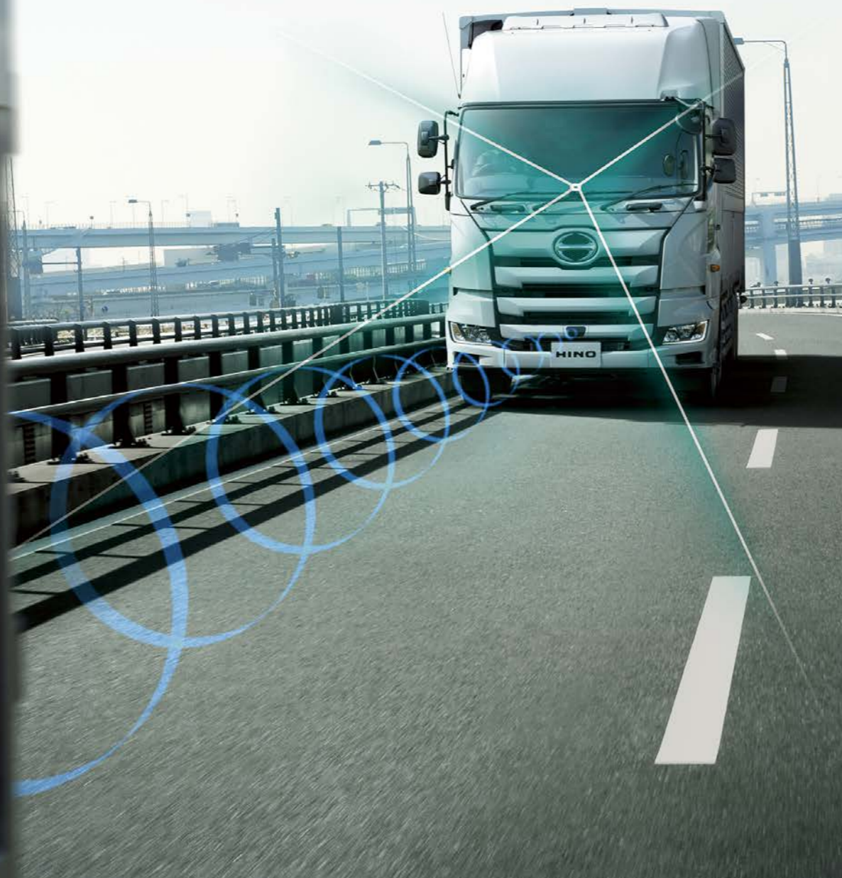
Pre-Crash Safety System (PCS)* (Collision Damage Reduction Brake) The PCS System utilizes millimeter wave radar and image sensors to detect vehicles and pedestrians ahead and automatically activates the brakes to reduce collision damage. Hino is installing this system as standard equipment on all truck models and large sightseeing buses. * PCS is a registered trademark of Toyota Motor Corporation.
